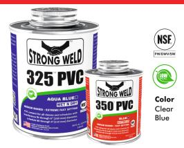
Fast setting PVC cement for all classes and schedules with interference fit through 6" (160 mm) diameter, schedule 80 through 4" (110 mm) diameter. Premium formula for wet conditions and/or quick pressurization.
